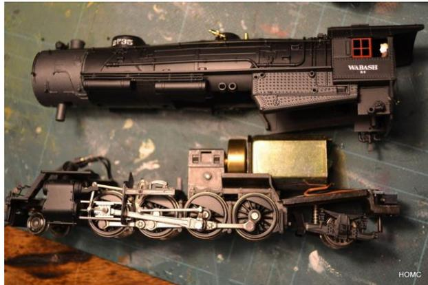
The approach of this modification is to give the impression of an M3s or M3as and the photos show that this is achieved without attention to minute detail. One main compromise is with check valves, which have been simulated with inverted stanchions where simulated at all. Others compromises are described at the end.
