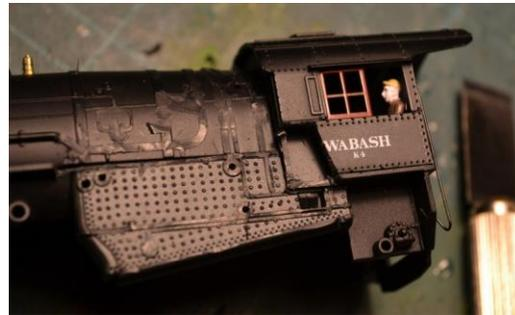
A similar treatment was given to the rest of the boiler, removing surface detail that was not wanted. This is a matter of taste – some details can be retained, but this makes it hard to get an even finish for adjacent parts – or the boiler can be left largely featureless with everything: pipework, boiler bands etc.. needing to be added fresh. In both cases, it is necessary to file after cutting, and then fill with green/white putty and finally sand with sanding sticks (purchased or home-made).
