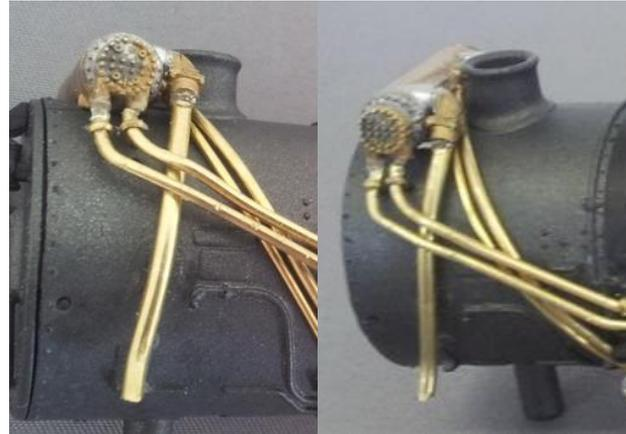
A slot was cut in the top of the smokebox to take the Feedwater heater using a razor saw (laterally) and drilled with an electric mini drill to make the ends of the slot. This results in a rectangular hole which disappears when the heater is placed in it.
