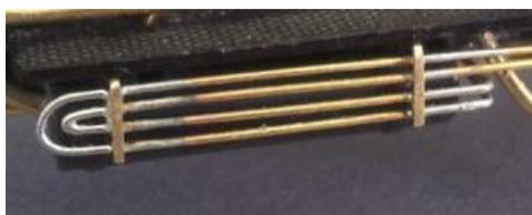
The cooling coils were scratch built from brass bar and wire and soldered together; a very rough jig was used for this. The brass bar extends up and is bent back and glued under the running board. In the picture above it can be seen that the wire is then extended to connect with the water pumps.
