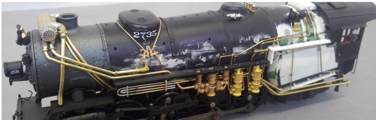
This larger picture of the finished LH side also shows the Cal-scale boiler check valve – the join to a piece of brass wire of the same diameter is hidden by an eyebolt and glued; Another eyebolt holds the end in position. The sander valves above it have been cut about and attached to the sand dome. Please also note the remaining white putty on the boiler after filling and sanding.
