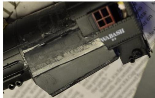
Layers of plastic-card were then added to build up the Wooton firebox shape as shown right. This required
