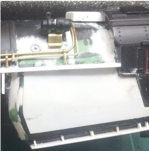
Further detailing around the cab/boiler area was also carried out with plastic card as shown right. Ash pans were added using superglue, as was a new running board and a safety-valve turret cover. The turret cover was pre-drilled, using a hand-held pin vice, to take the pipework (wire).
