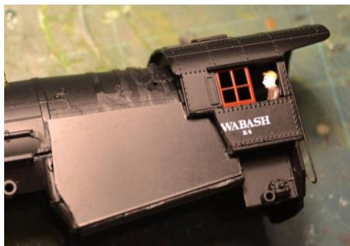
Meanwhile, back to the firebox, a sheet of black plastic-card was cut to the desired shape and glued to the firebox side with polystyrene cement – to fill some of the gaps underneath.
