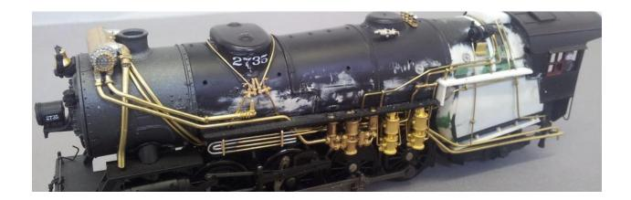
The cooling coils were scratch built from brass bar and wire and soldered together by Richard Oldfield; a very rough jig was used for this. The brass bar extends up and is bent back and glued under the running board. In the picture above it can be seen that the wire is then extended to connect with the water pumps.
