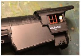
A similar treatment was given to the rest of the boiler, removing surface detail that was not wanted. This is a matter of taste – some details could be retained, but his makes it hard to get an even finish for adjacent parts – or the boiler can be left largely featureless with everything: pipework, boiler bands etc.. needing to be added fresh. In both cases, it is necessary to file after cutting, and then fill with green/white putty and finally sand with sanding sticks
